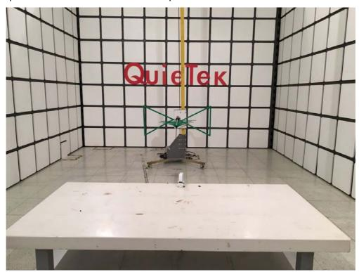
Description: Radiated Emission Test Setup for 1~18GHz
