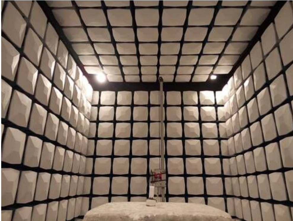
Test Mode: TransmitDescription: Front View of Radiated Emission Test Setup for Above 1GHz
