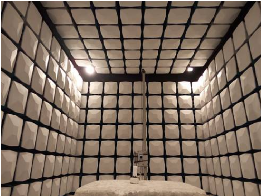
Test Mode: TransmitDescription: Front View of Radiated Emission Test Setup for Above 18GHz
