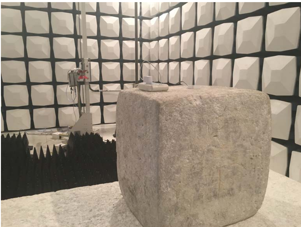
Description: Radiated Emission Test Setup for 1~18GHz
