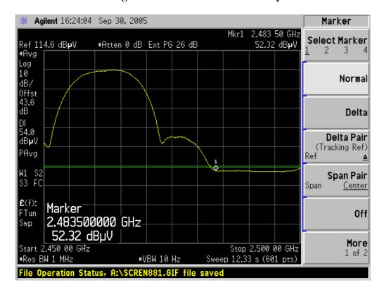
Detector mode: Peak Polarity: Horizontal
