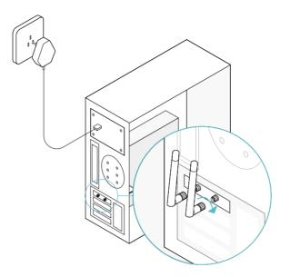
4. Replace the case panel, plug in the power cable and turn on your computer.
