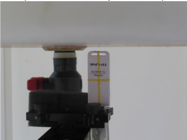
USB Cable Plug-in for USB Configuration 5 (Tip Mode, Test Separation 5 mm)
