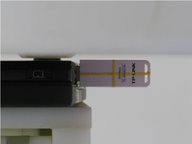
Direct Laptop Plug-in USB Configuration 3 (Vertical Front, Test Separation 5 mm)
