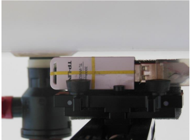
USB Cable Plug-in for USB Configuration 4 (Vertical Back, Test Separation 5 mm)
