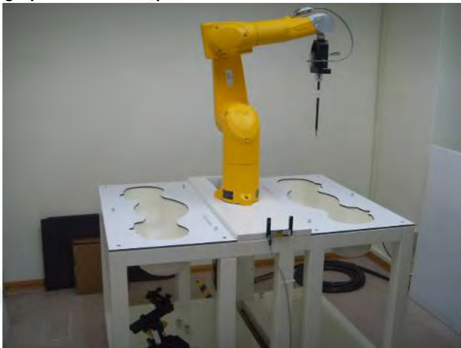
Fig.1 Photograph of the SAR measurement System
