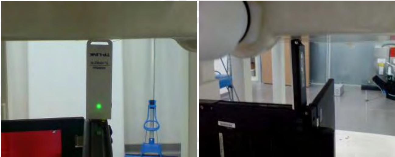
Fig.7 Tip of EUT is paralleled with flat phantom, and contact it.
