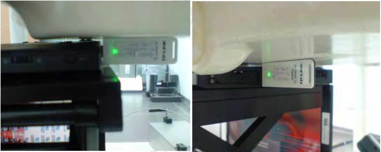
Fig.5 Bottom side of the Notebook is paralleled and contacted with flat phantom, and left side of the EUT is paralleled with flat phantom.
