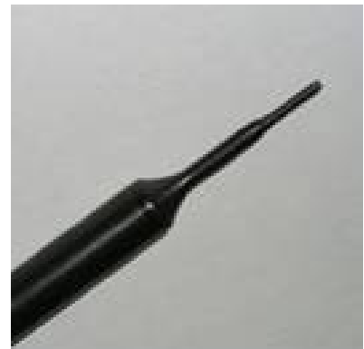
Figure 2. EX3DV4 E-field Probe
