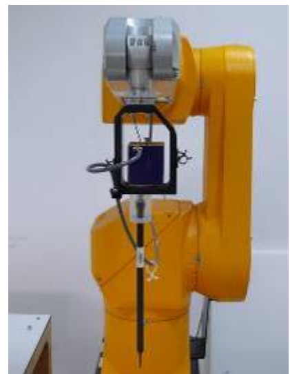
Figure 3. EX3DV4 E-field probe
