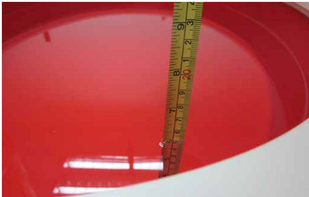
Figure 4.4: Liquid depth in the Flat Phantom
