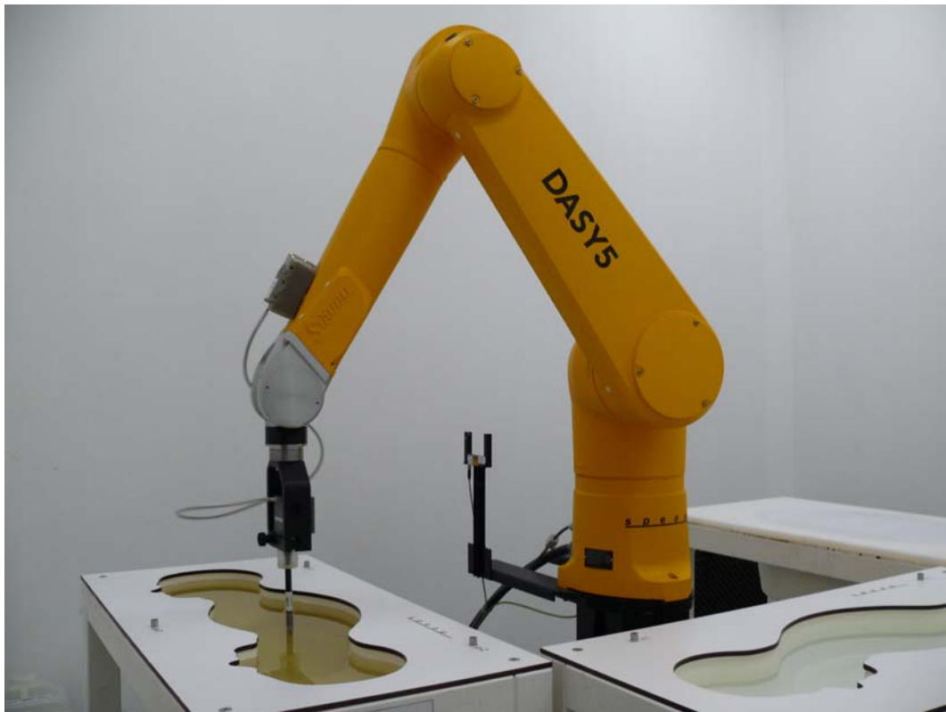
Picture 2: Specific Absorption Rate Test Layout
