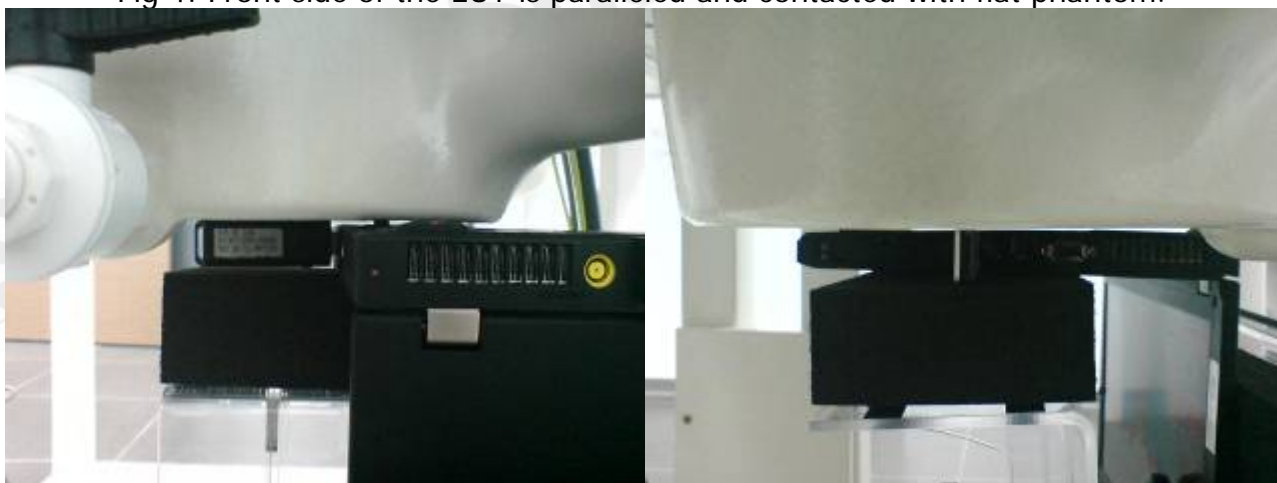
Fig 5 : Bottom side of the Notebook is paralleled and contacted with flat phantom, and left side of the EUT is paralleled with flat phantom.
