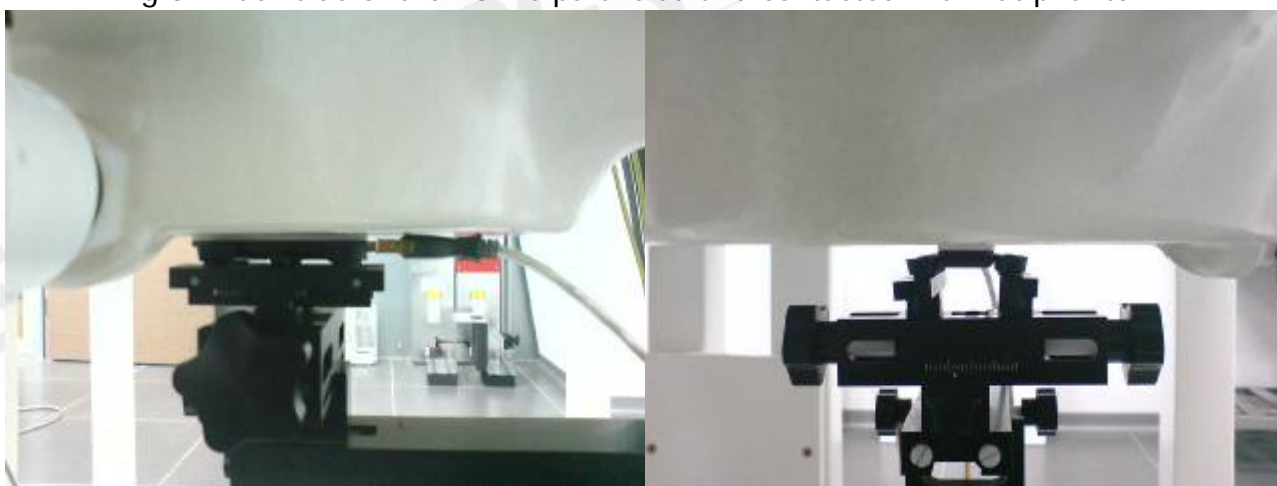
Fig 4: Front side of the EUT is paralleled and contacted with flat phantom.
