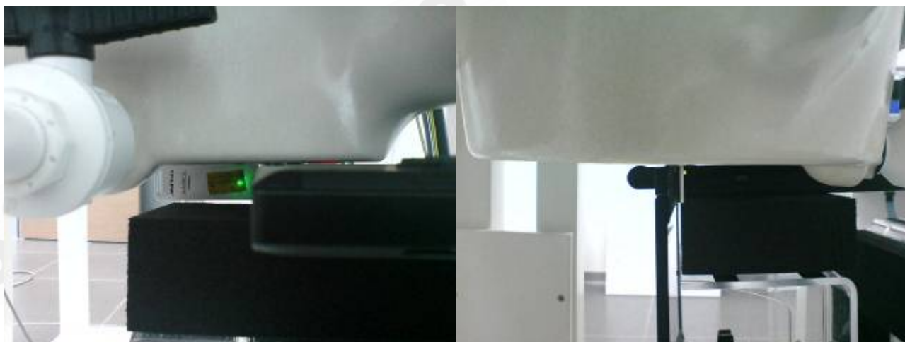
Fig 6 : Bottom side of the Notebook is paralleled and contacted with flat phantom, and right side of the EUT is paralleled with flat phantom.
