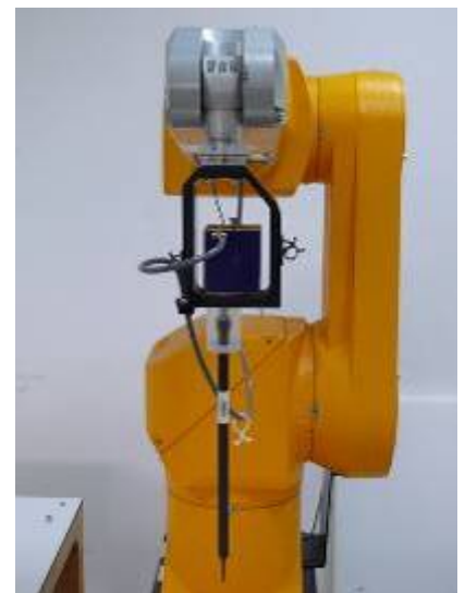
Figure 3. EX3DV4 E-field probe
