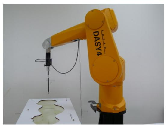
Picture 2: Specific Absorption Rate Test Layout
