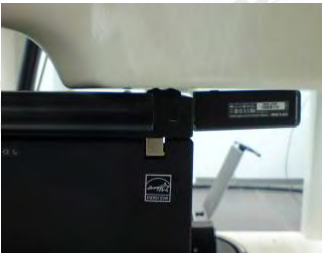
Fig.6 Bottom side of the Notebook is paralleled and contacted with flat phantom, and right side of the EUT is paralleled with flat phantom.
