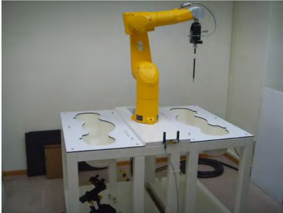
Fig.1 Photograph of the SAR measurement System
