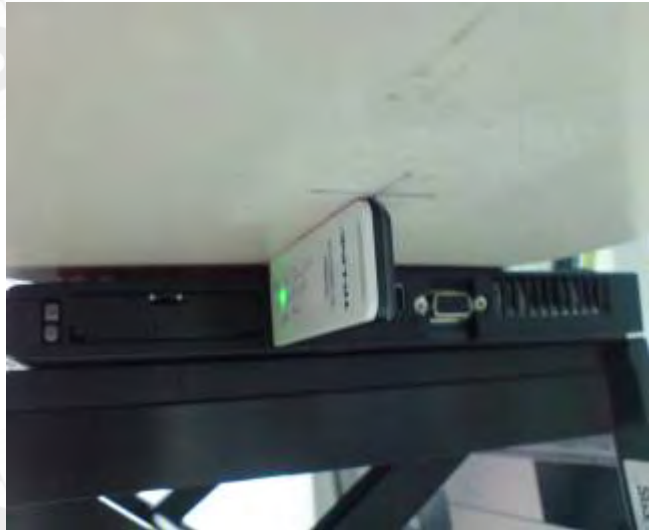
Fig.5 Bottom side of the Notebook is paralleled and contacted with flat phantom, and left side of the EUT is paralleled with flat phantom.
