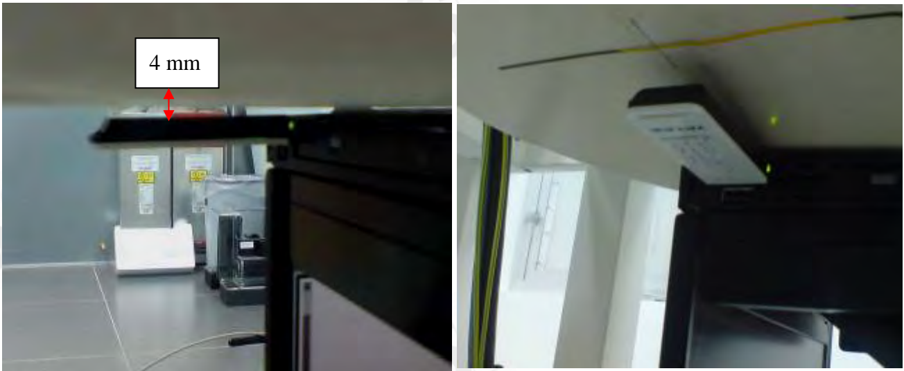
Fig.3 Back side of the EUT is paralleled with flat phantom, and spacing between EUT and Phantom is 4 mm.
