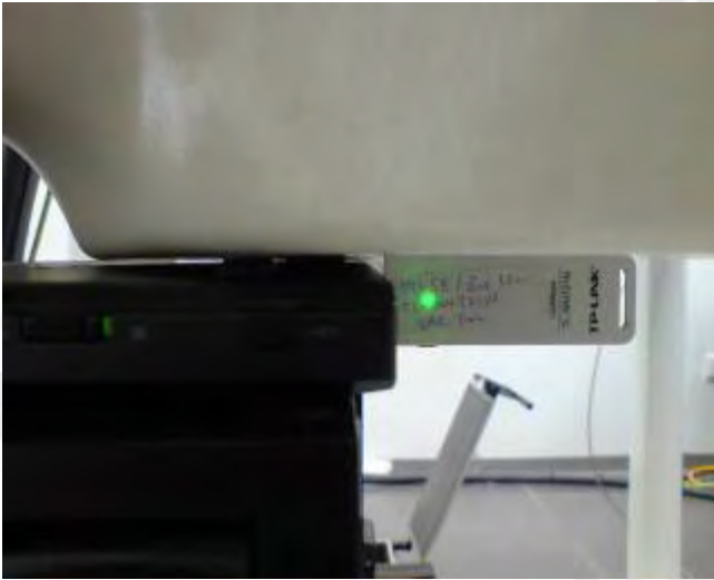
Fig.5 Bottom side of the Notebook is paralleled and contacted with flat phantom, and left side of the EUT is paralleled with flat phantom.
