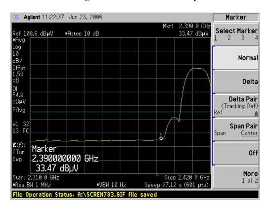
Detector mode: Peak Polarity: Horizontal
