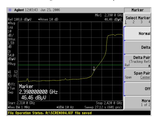
Detector mode: Peak Polarity: Horizontal
