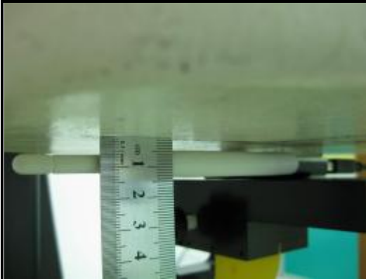
D. The front of the EUT face to the phantom with 5mm-separation distance. (Antenna degree: 180°)
