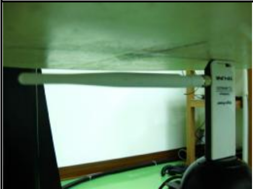
F. The tip of the EUT face to the phantom with 0mm-separation distance. (Antenna degree: 90°)
