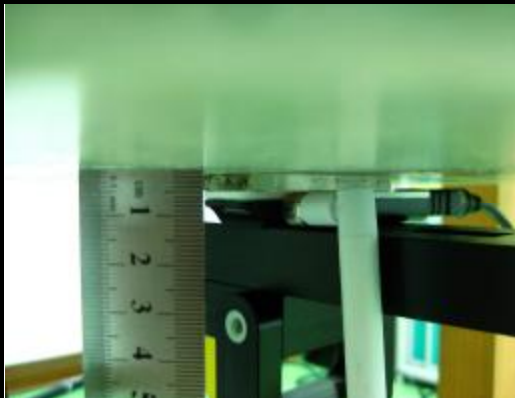
E. The front of the EUT face to the phantom with 5mm-separation distance. (Antenna degree: 90°)
