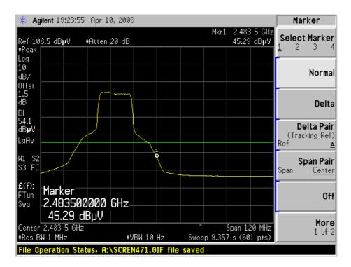
Detector mode: Peak Polarity: Horizontal
