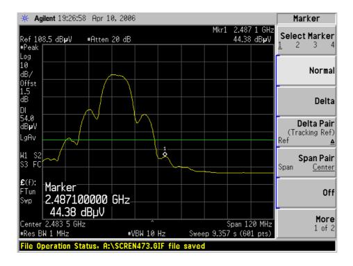
Detector mode: Peak Polarity: Horizontal
