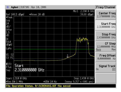
Detector mode: Peak Polarity: Horizontal
