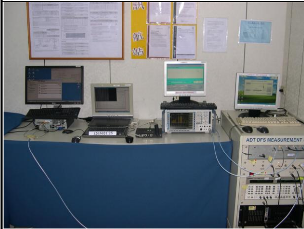
EUT (Client ) links with master on 5310MHz
