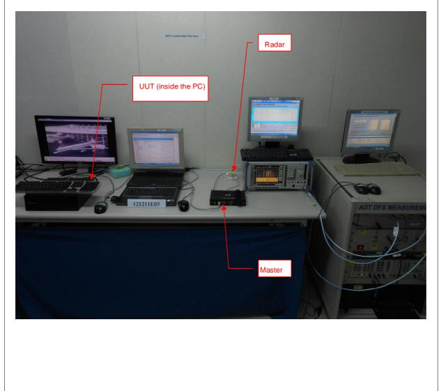
Set UUT as Client without radar detection mode (Radar injected into Master)
