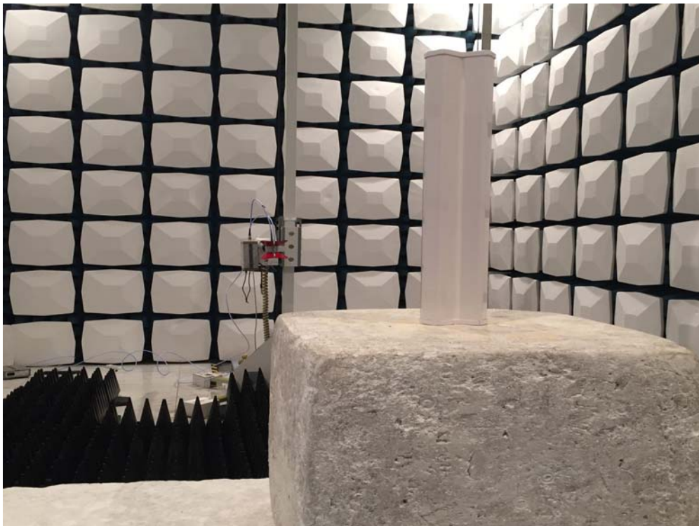
Description: Radiated Emission Test Setup for 1~18GHz
