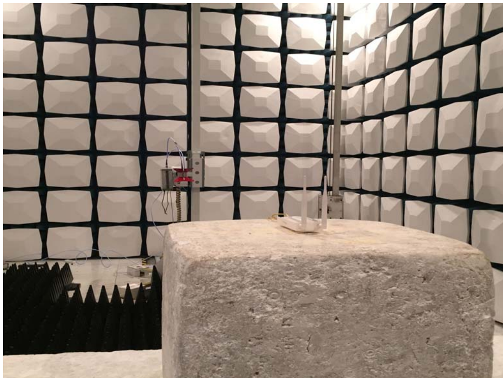
Description: Radiated Emission Test Setup for 1~18GHz
