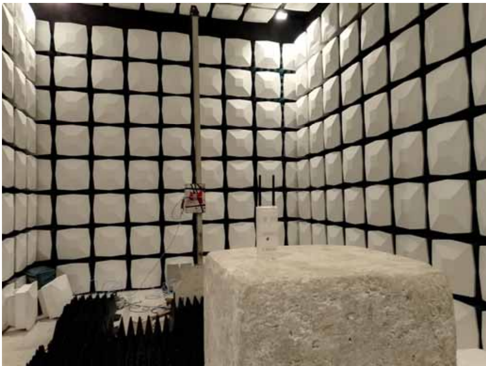
Description: Radiated Emission Test Setup for 1~18GHz
