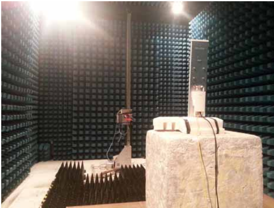
Description: Radiated Emission Test Setup for 1~18GHz
