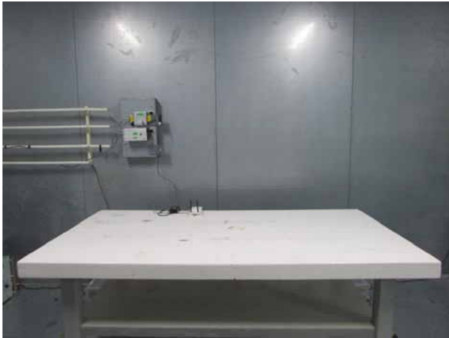
Description: Conducted Emission Test Setup
