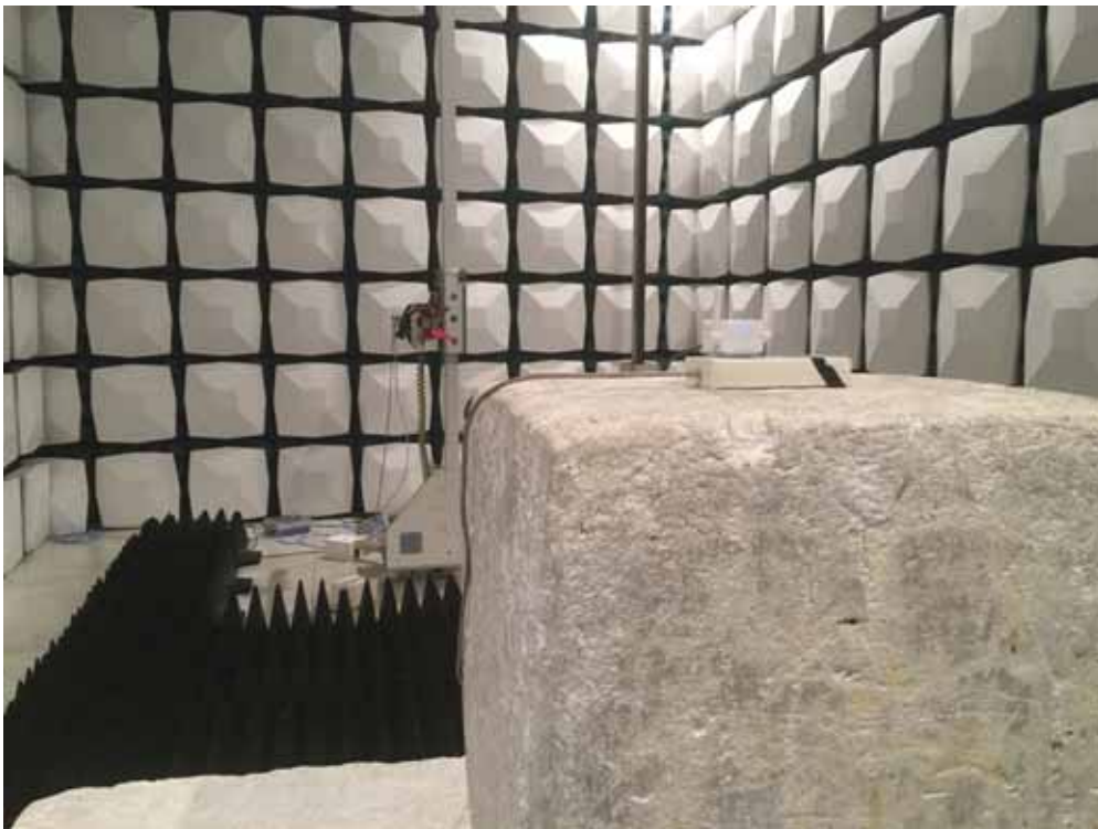
Description: Radiated Emission Test Setup for 1~18GHz
