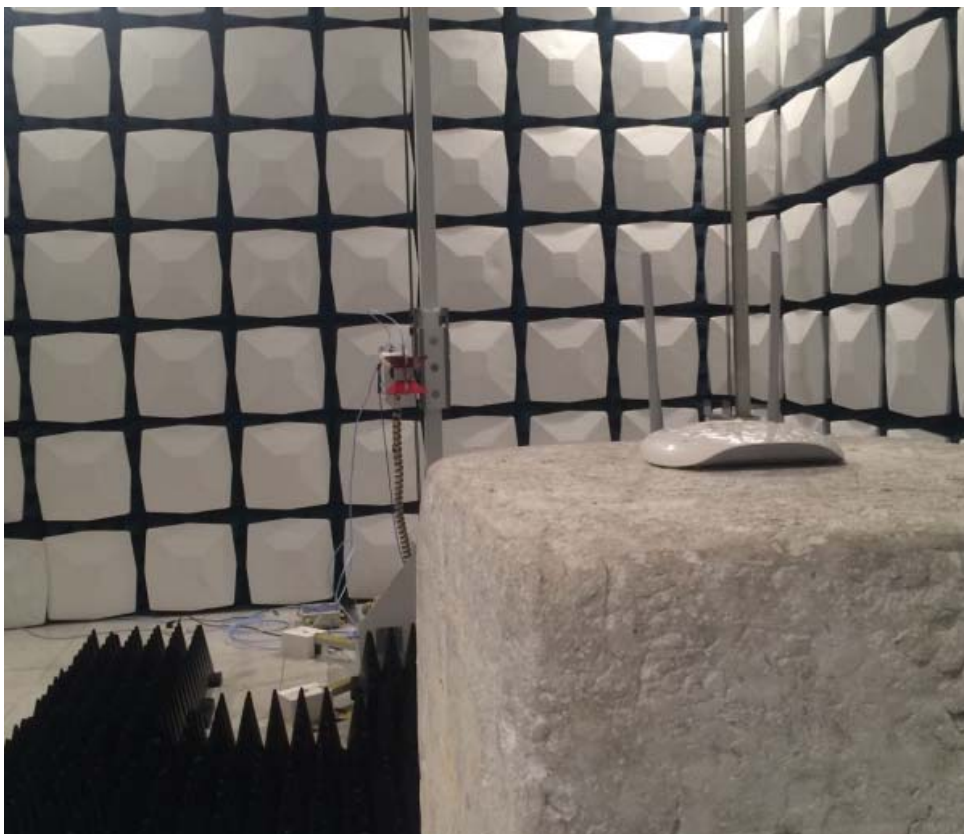
Description: Radiated Emission Test Setup for 1~18GHz
