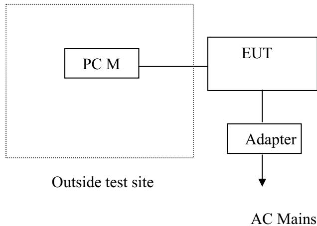
(EUT: 150Mbps Wireless N ADSL2 + Modem Router)
