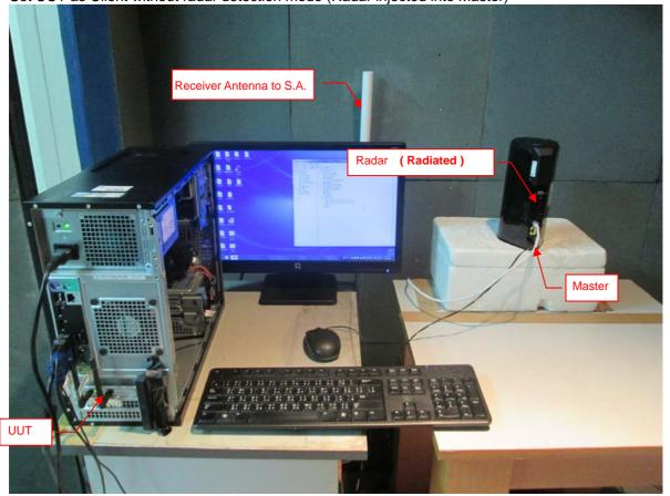
Set UUT as Client without radar detection mode (Radar injected into Master)
