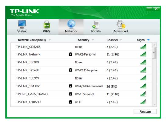
2. Select the network you want to join from the list on this screen and click Connect. If you want the adapter to automatically connect to the network next time, select the Connect automatically checkbox. Enter your Wi-Fi password when prompted.
