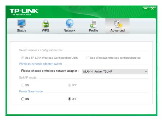
Select wireless configuration tool: In Windows XP, you can either use TP-LINK Utility or Windows wireless configuration tool. While in other operating systems, since you can use both TP-LINK Utility and Windows wireless configuration tool at the same time, this function is disabled.
