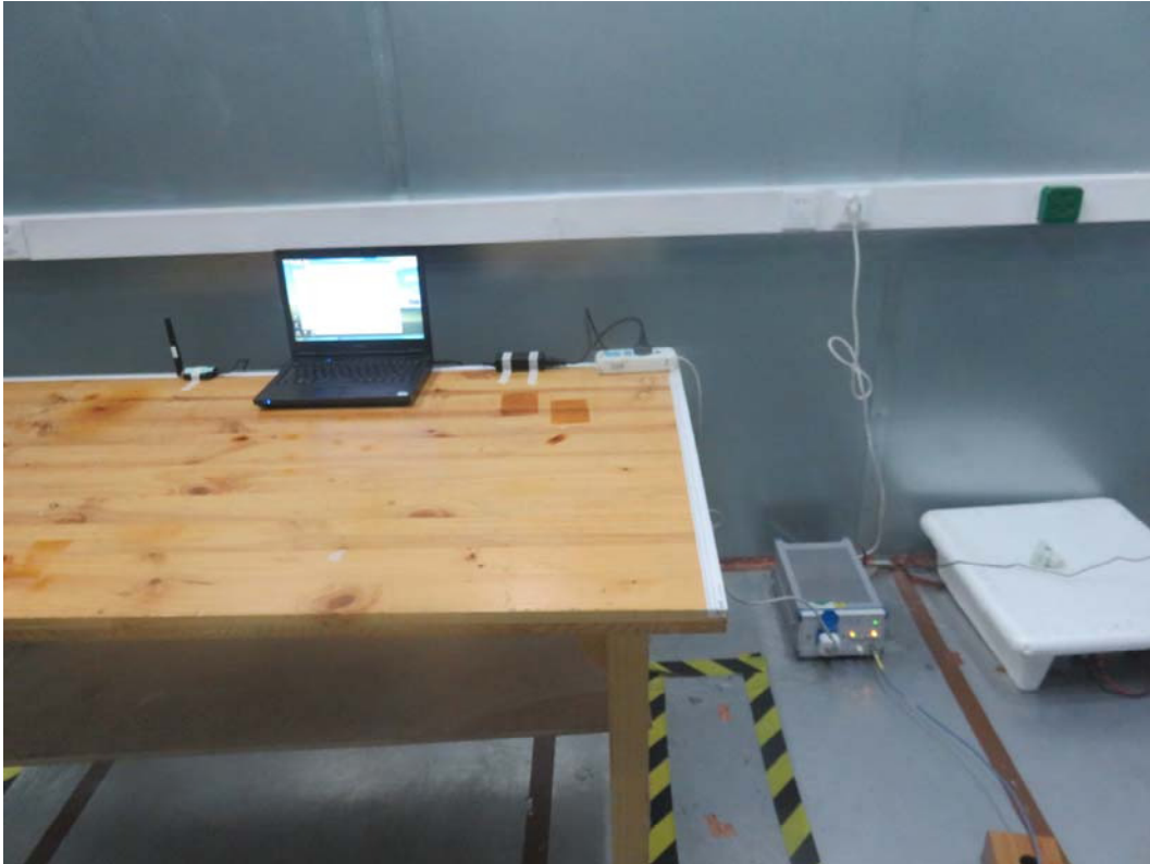
Picture 3 Conducted Emission Test Setup
