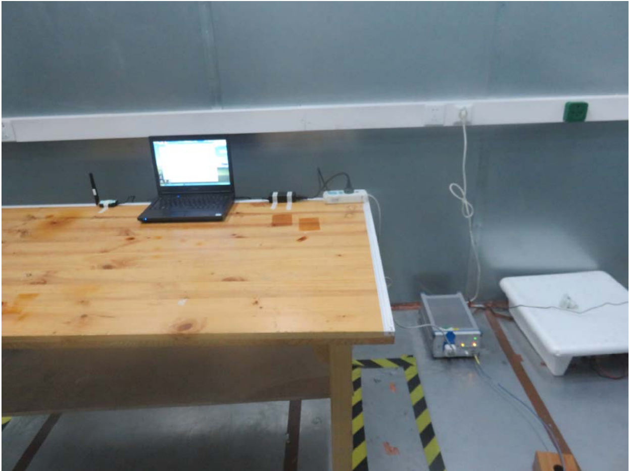
Picture 3 Conducted Emission Test Setup
