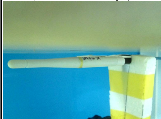
Test Position 3: USB Horizontal Down with 0.5 cm gap (Antenna in vertical at 180 degree)
