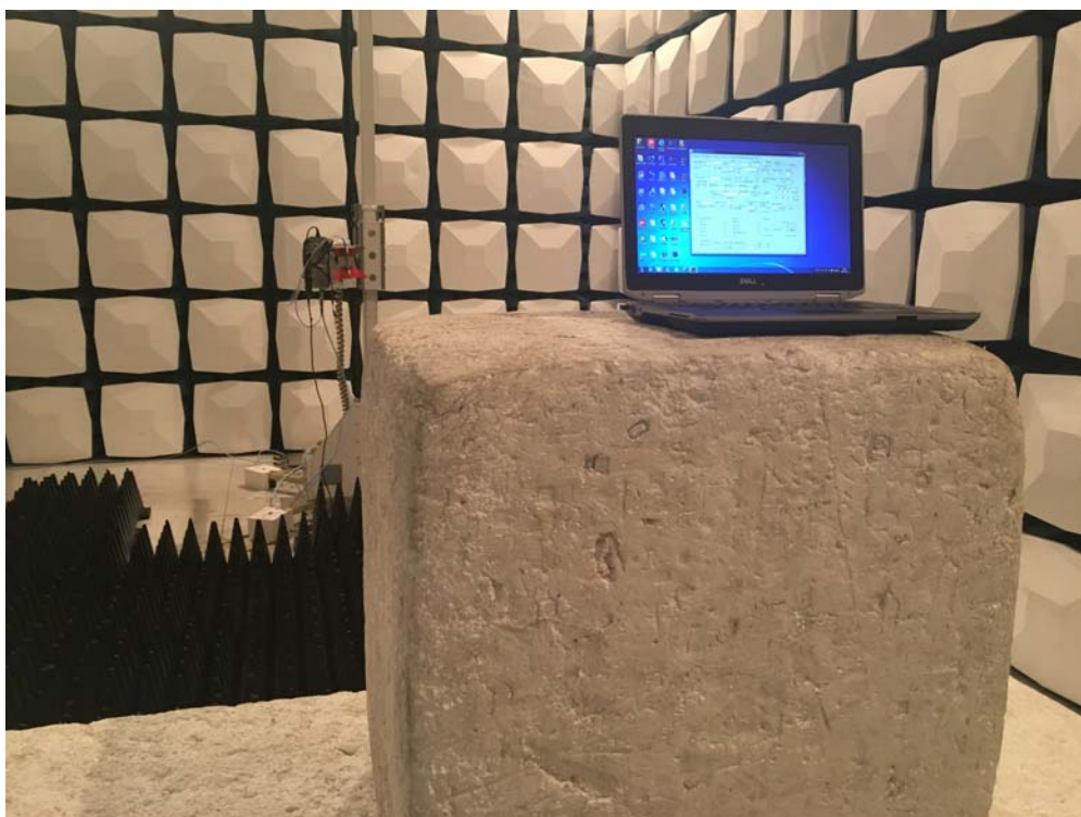
Description: Radiated Emission Test Setup for 1~18GHz
