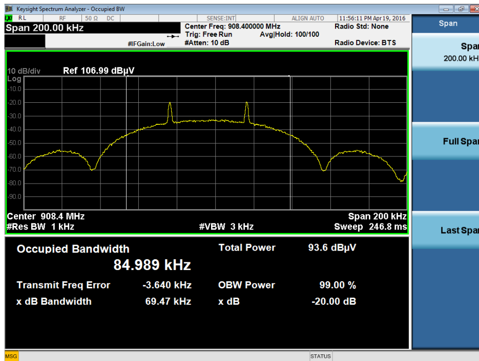
20 dB and 99% Occupied Bandwidth Plot on 40 kbps
