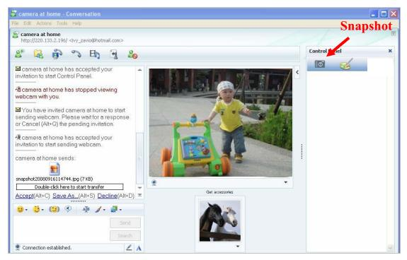
14. You can click paint palette icon showing up with tool bar to set up image. Then, you can use the tool bar to optimize video Brightness , Contrast , Saturation and Hue . After the adjustment of all setting, you can still click Default to make the setting back to the original setting.
