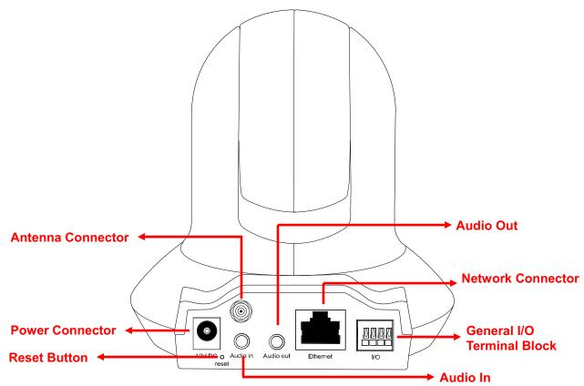
Power Connector: For connection of 12V DC input.
