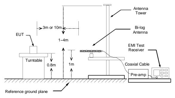
The diagram below shows the test setup that is utilized to make the measurements for emission above 1GHz.
