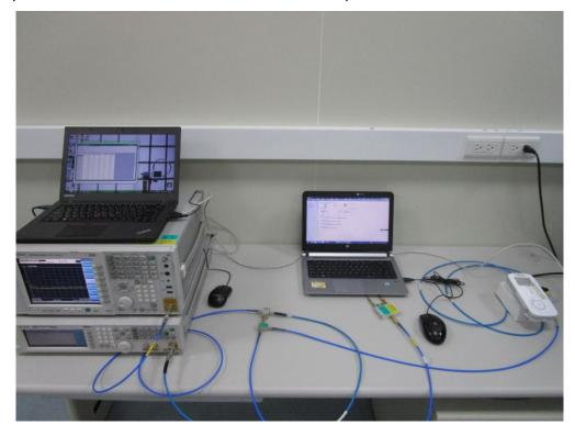
Description: DFS Radiated Measurement Test Setup
