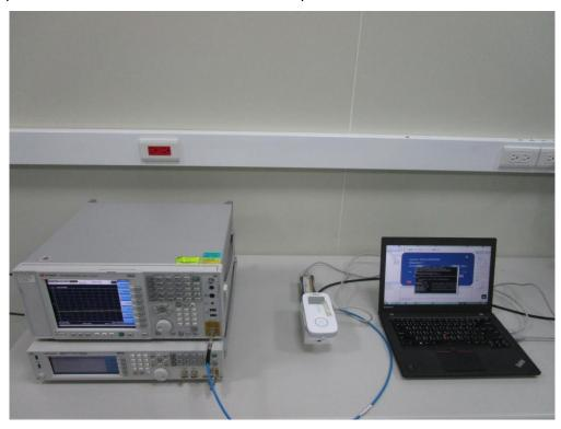
Description: DFS Conducted Measurement Test Setup
