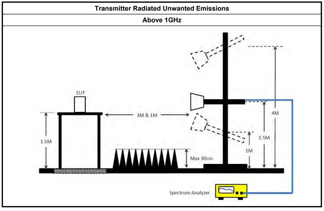
3.4.5 Test Result of Transmitter Unwanted Emissions
