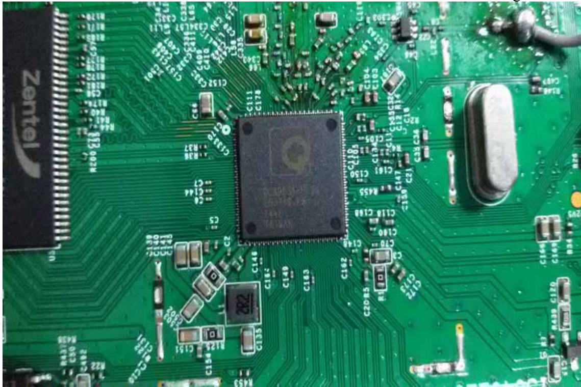
Figure 15 Inside Configuration of the EUT
