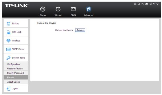
Figure 4-31 Reboot the Device
