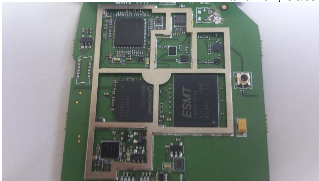
Photo 10 Internal View (2G & 3G Module)
