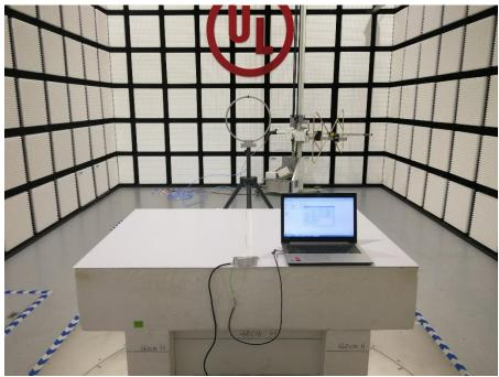
POWERLINE CONDUCTED EMISSIONS MEASUREMENT SETUP
