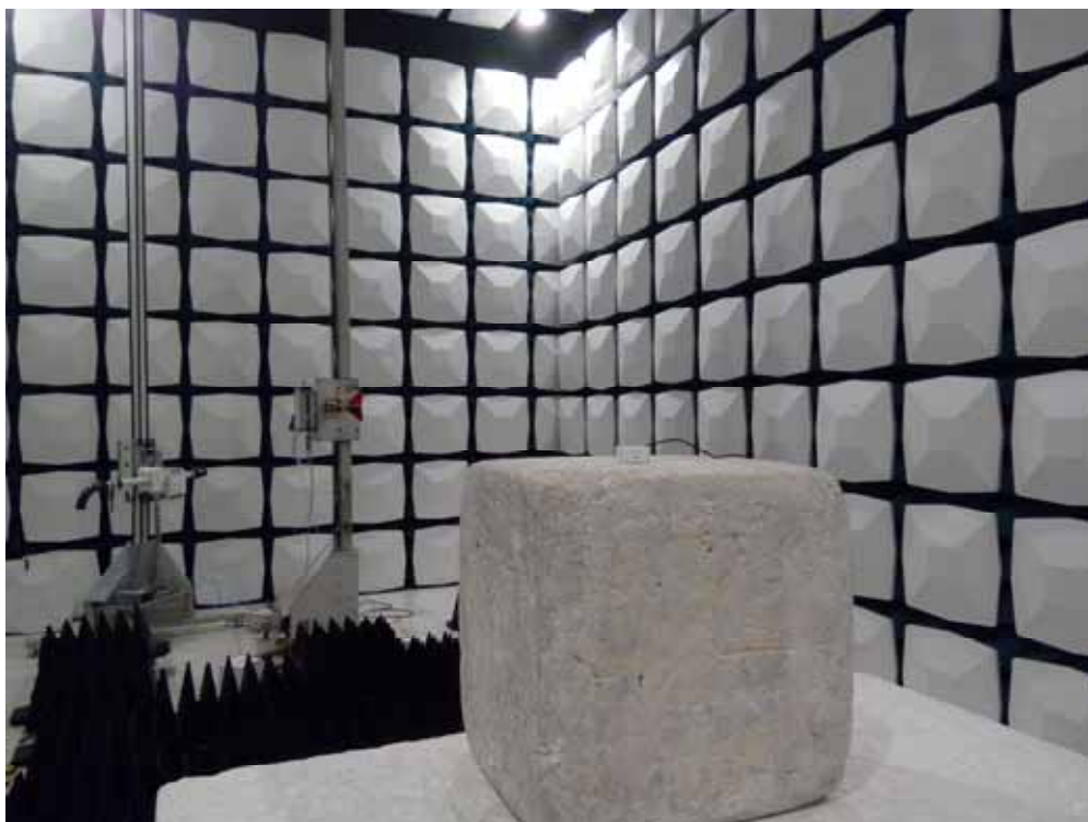
Description: Radiated Emission Test Setup for 1~18GHz
