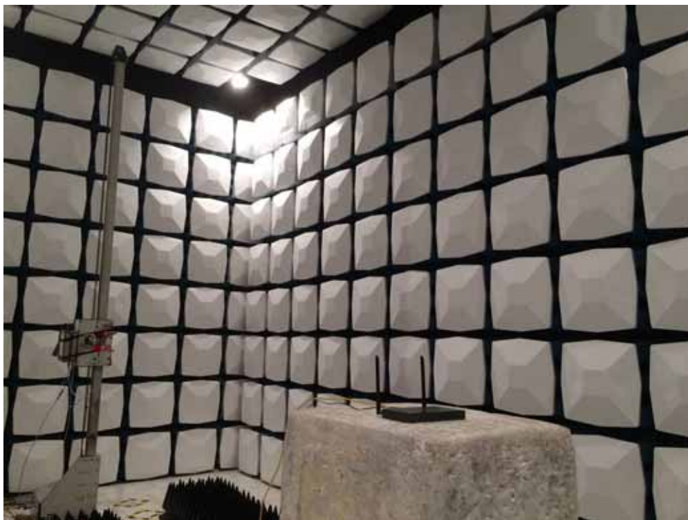
Description: Radiated Emission Test Setup for 1~18GHz
