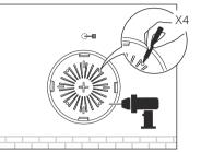
If your Ethernet cable feeds through the wall, you can position the mounting bracket below the cable hole. Mark four positions for the screw holes and then drill four 6 mm diameter holes at the marked positions
