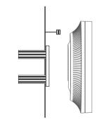
Connect the Ethernet cable to the Ethernet port on the EAP
