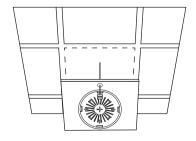
Feed the Ethernet cable through the hole and set the ceiling tile back into place.
