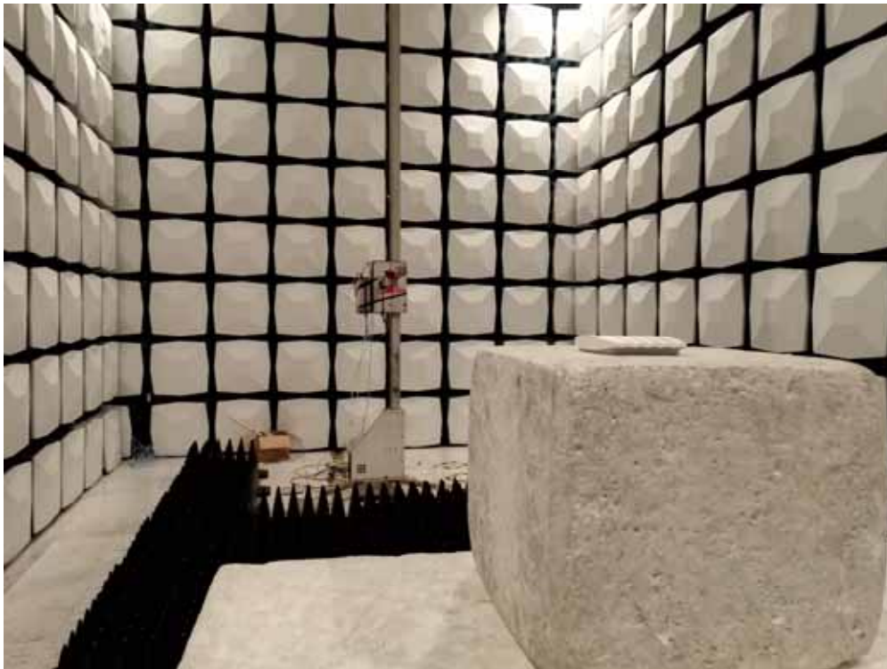
Description: Radiated Emission Test Setup for 1~18GHz
