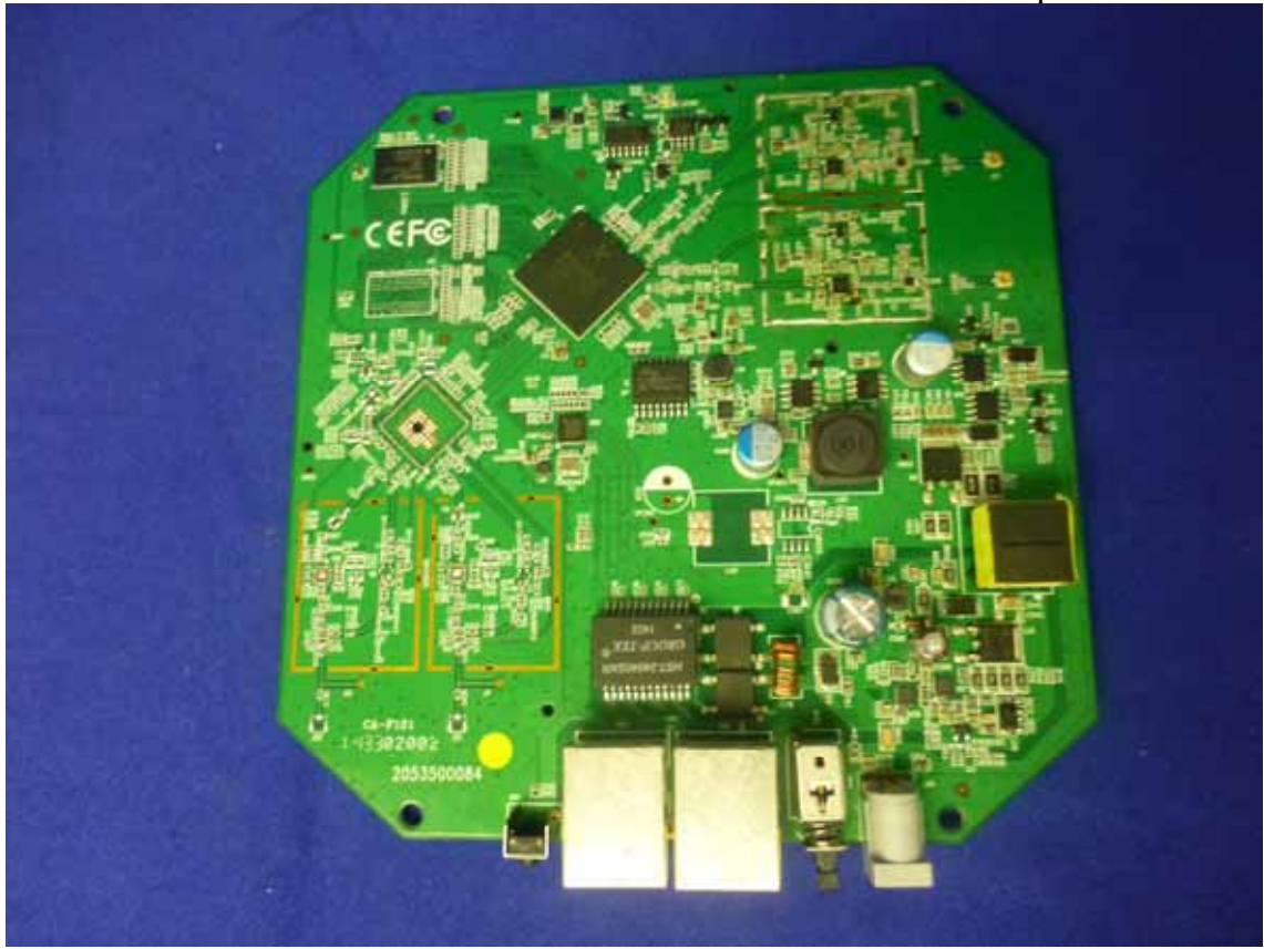
Figure 8 Components Side of the PCB
