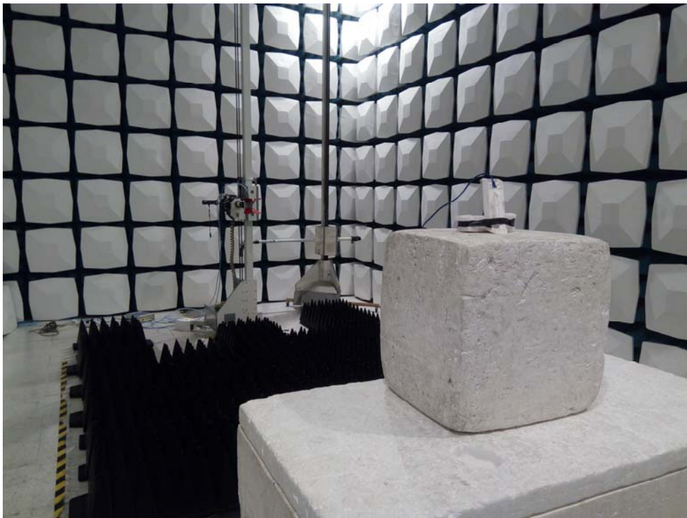
Description: Radiated Emission Test Setup for 1~18GHz
