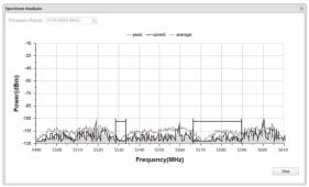
4. Close the Spectrum Analysis Window, and then you will get back to the Wireless page. For the Channel/Frequency option, it is recommended to select a value whose frequency is within the noted frequency range.
