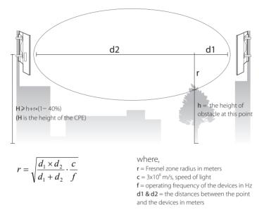
For example, assume d1 is 2km, d2 is 8km, and f is 2.4GHz, then r would be 14.142m. Considering a toleration of 40%, allowable radius would be 8.485m. Assume h is 10m, then the result of the minimum mounting height based on this point would be 18.485m. Similarly, calculate the results based on all the points where there are obstacles, and the maximum value would be the final result.
