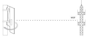
Adjust the direction of the CPE until the device reaches the highest SNR
