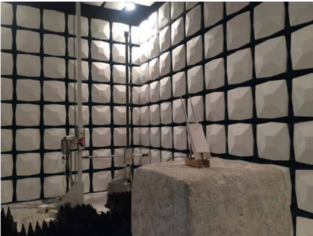
Description: Radiated Emission Test Setup for 1~18GHz
