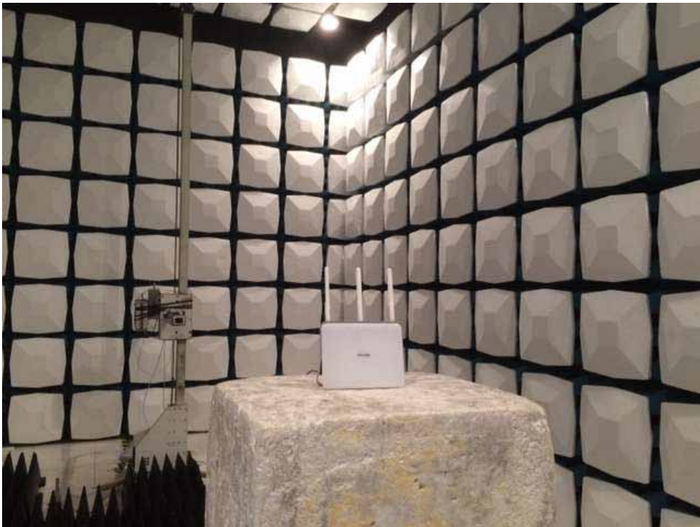
Description: Radiated Emission Test Setup for 18~40GHz
