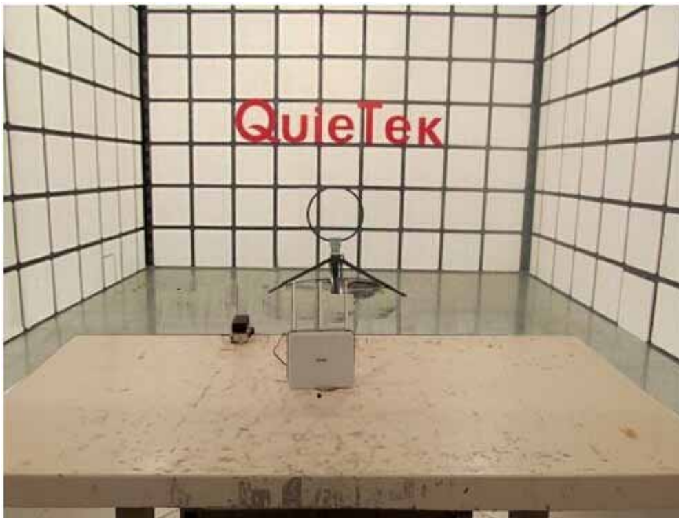
Description: Radiated Emission Test Setup for Below 30MHz
