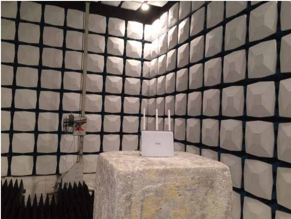
Description: Radiated Emission Test Setup for 1~18GHz
