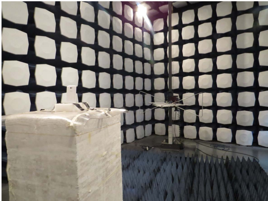
Picture 2 Radiated Spurious Emissions Test Setup
